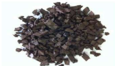
Fig 2.1 Chipped rubber tyre of size 20mm
