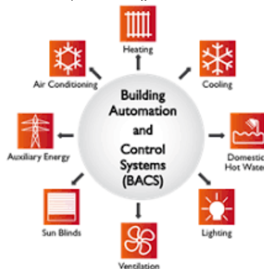
Fig 1.1 Building Automation and Control Systems
