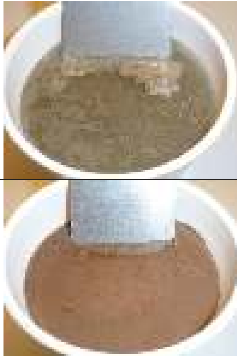
Figure 1: Aluminium metal plate placed in OPC paste (top) evolving gas and in paste where OPC is replaced with 50% calcined marl (bottom).
