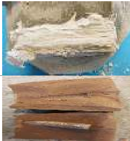
Figure 2: Al/5% Mg alloy rods placed in OPC paste (top) and totally converted to gibbsite after 28 days curing in moist condition, while same rod placed in paste where OPC is replaced with 55% calcined marl is in pristine condition without any corrosion products in its imprint (bottom).
