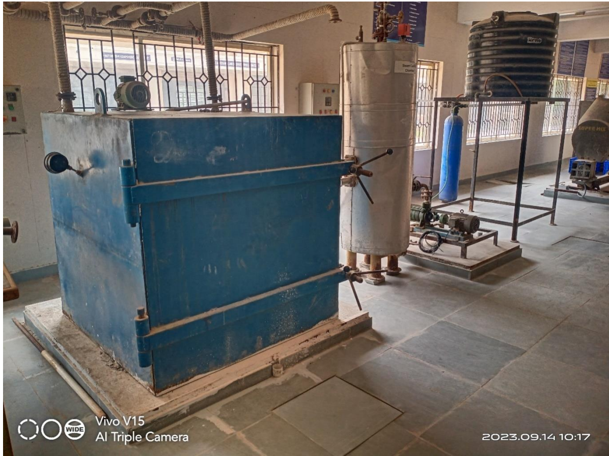
Steam Curing Chamber
